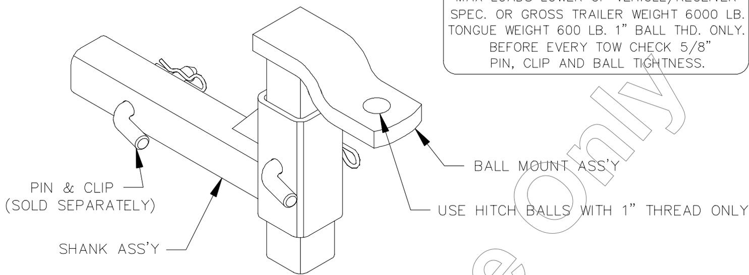
1. INSERT SHANK ASS'Y INTO HITCH RECEIVER AND ATTACH PIN & CLIP (SOLD SEPARATELY).
