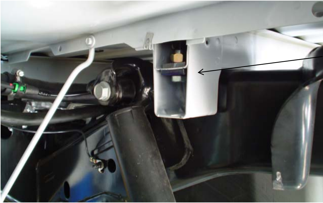
CUT HERE, BELOW THE MAIN HAT CHANNEL, TO REMOVE THE LOWER EXTENSION IF MORE ACCESS SPACE IS NEEDED.
